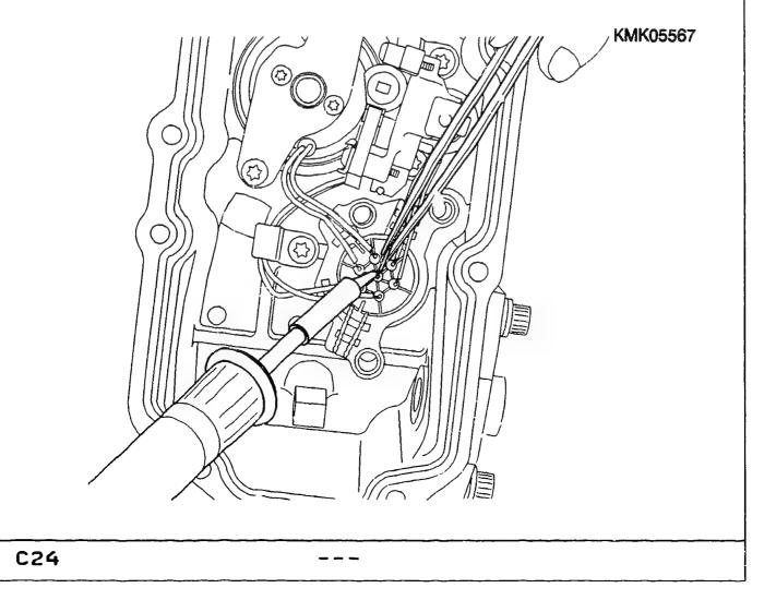
New components are supplied with correct length of lead and with crimped-on soldering eyes. Changes to the leads are not permitted.
